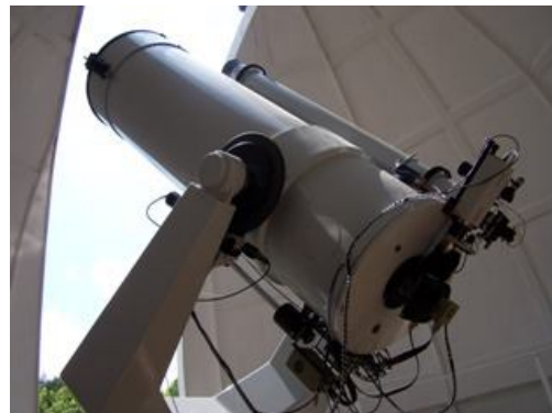
II TNT telescope (Teramo Normal Telescope) with a diameter of 72 cm.
