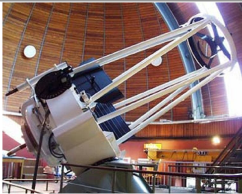
The Ruths 134cm telescope used for the observations of the GJ436b transit.
